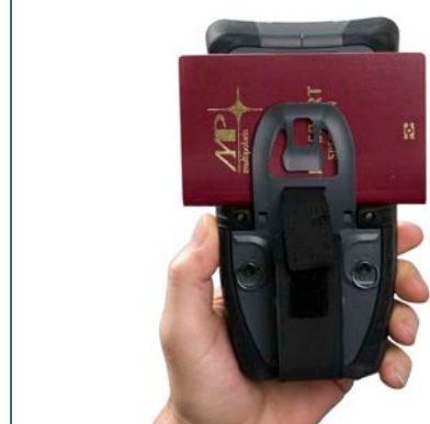
A convenient clip holder allows one handed operation while the Be.U e-Passport reads electronic chips.
