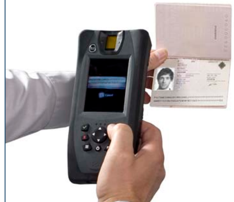
The Be.U e-Passport camera enables users to read MRZ data without swiping the document.
